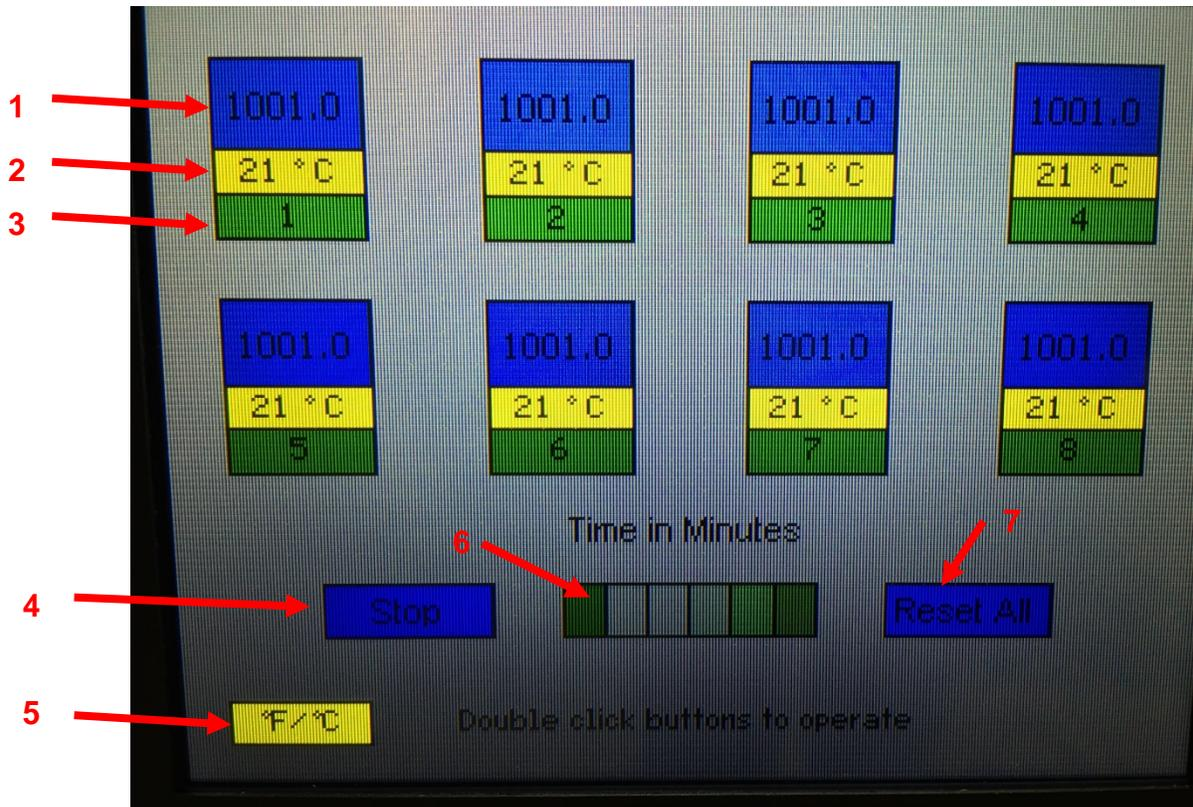
1. **TIME DISPLAY:** Displays time in minutes. Double clicking a Test Bank's Time Display will reset the time to zero for that Test Bank.
