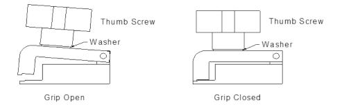
NOTE: The grip is attached directly to the load cell. Do not move the grip sideways or up and down. When opening and closing the grip, support it with one hand and operate the thumb screw with the other hand to avoid damaging the load cell. For proper operation of the load cell it is necessary for the grip to be mounted with a space between the load cell housing and the grip. DO NOT TIGHTEN THE GRIP AGAINST THE LOAD CELL HOUSING.
