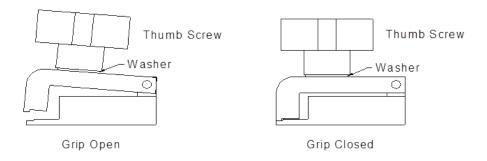
NOTE: The grip is attached to the load cell through the yoke by the mounting pin. Remove the grip from the Load Cell Assembly to load samples into the grip.
