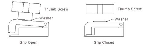
NOTE: The grip is attached directly to the load cell. Do not move the grip sideways or up and down. When opening and closing the grip, support it with one hand and operate the thumb screw with the other hand to avoid damaging the load cell. For proper operation of the load cell it is necessary for the grip to be mounted with a space between the load cell housing and the grip. DO NOT TIGHTEN THE GRIP AGAINST THE LOAD CELL HOUSING.
