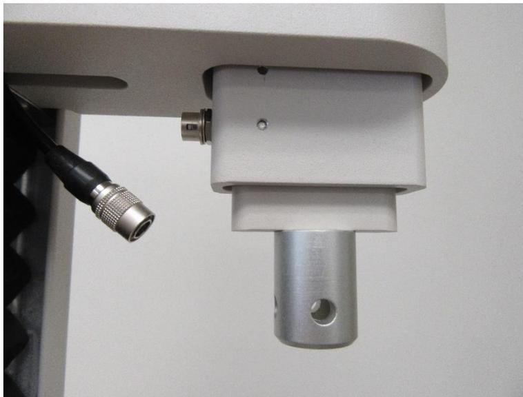
3. Remove the screw from the top of the load cell assembly. **Make sure that you support the load cell so that it does not fall.**
