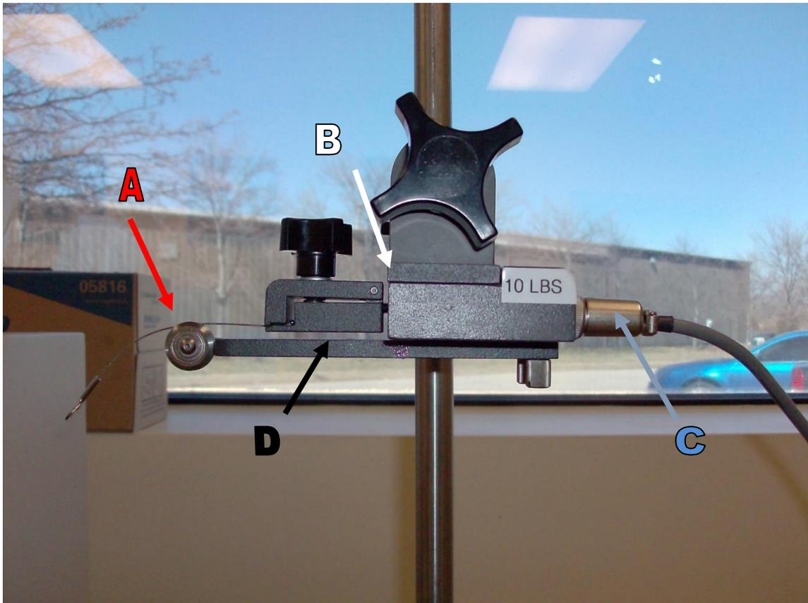
A: Be sure that the calibration wire is in the groove running through the center of the bearing.
