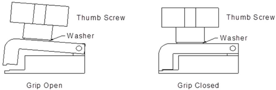
**NOTE:** The grip is attached directly to the load cell. Do not move the grip sideways or up and down. When opening and closing the grip, support it with one hand and operate the thumb screw with the other hand to avoid damaging the load cell. For proper operation of the load cell it is necessary for the grip to be mounted with a space between the load cell housing and the grip. **DO NOT TIGHTEN THE GRIP AGAINST THE LOAD CELL HOUSING.**
